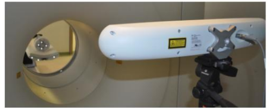
Fig. 3. Motion tracking setup for a CT on a Siemens Biograph 16 PET/CT scanner. This figure is from [20].
